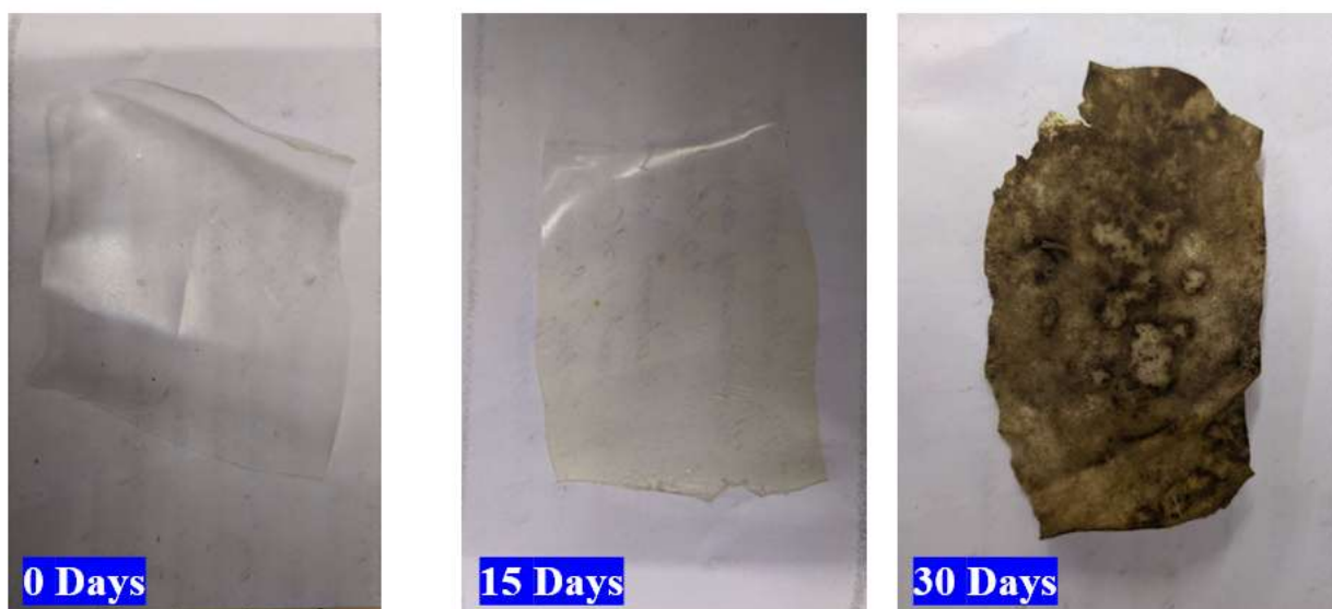
Figure 1. Starch-based film samples before and after soil exposure
