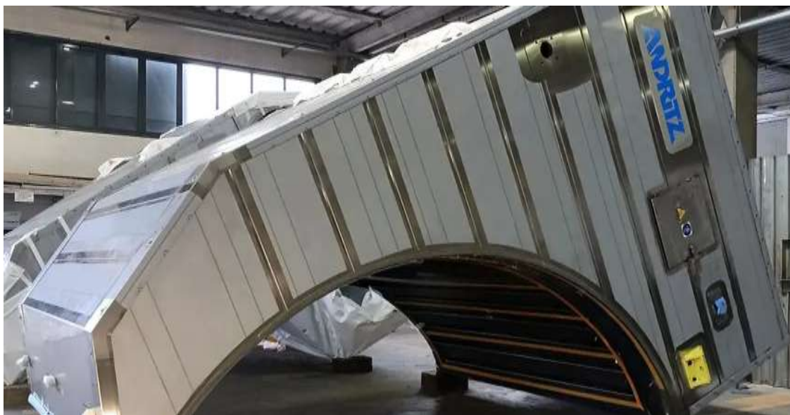
Figure 4 - Yankee cylinder with the PrimeDry cap [7]
