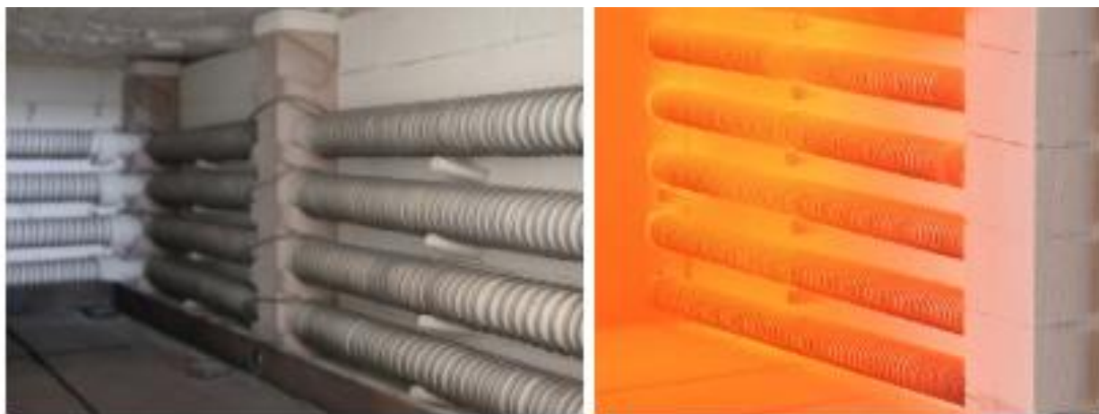
Figure 2 – Heating elements of the chamber furnace
