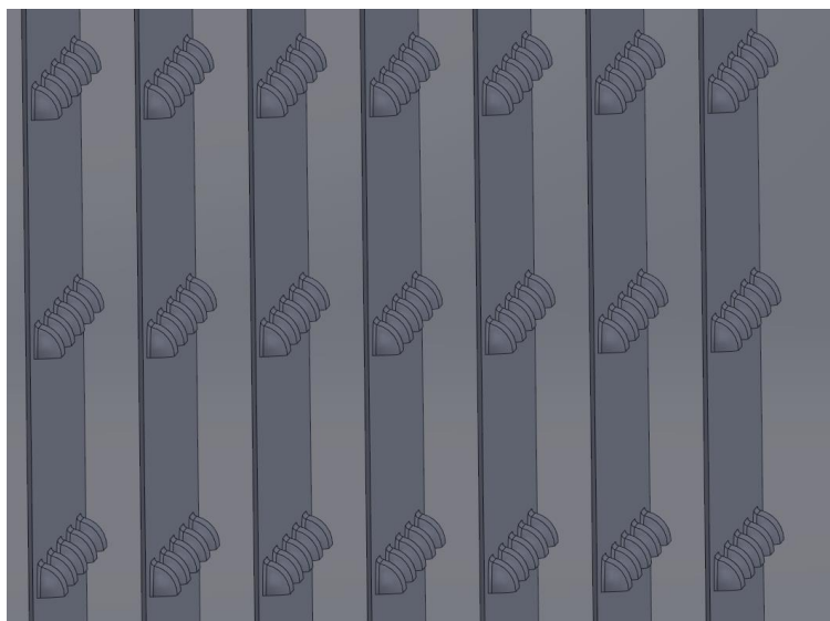
Figure 3 – modernized plates in the heat exchanger
