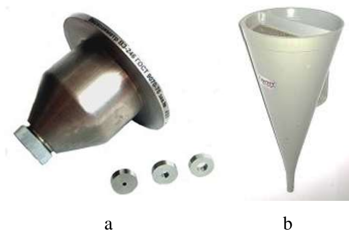
Figure 1. Flow-through cup viscometer with a set of nozzles (a) and Marsh funnel (b)
